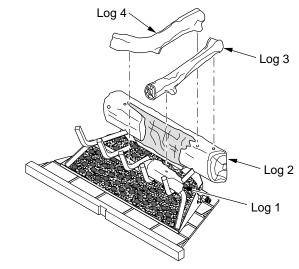
Figure 26 - Installing Logs 3 and 4
